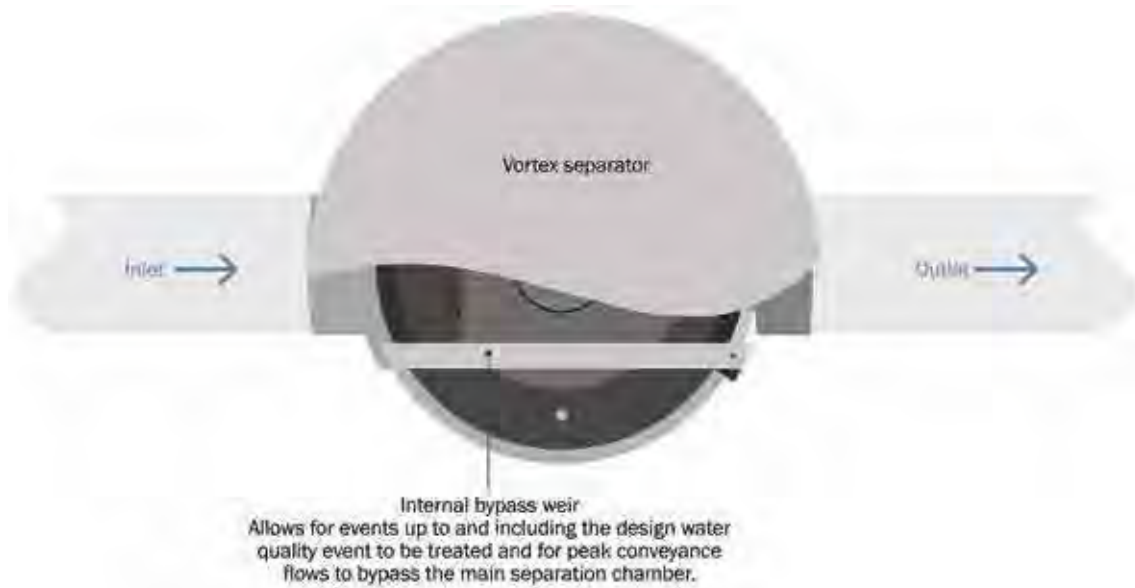
Figure 14.6 Hydrodynamic separator with an internal (or integral) bypass (courtesy Hydro International)
