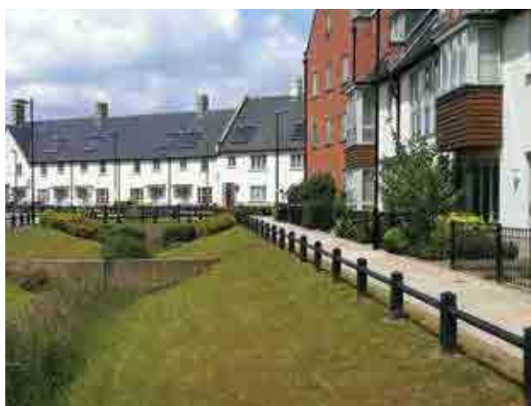
Figure 17.8 Dry swale with overlying flow control, Upton, Northamptonshire (courtesy Peterborough City Council)
